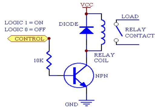
Fig -4: Relay Driver Circuit
