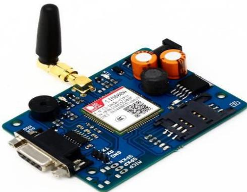
Fig -6: GSM Module
