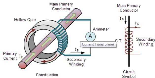
Fig -3: Current Transformer
